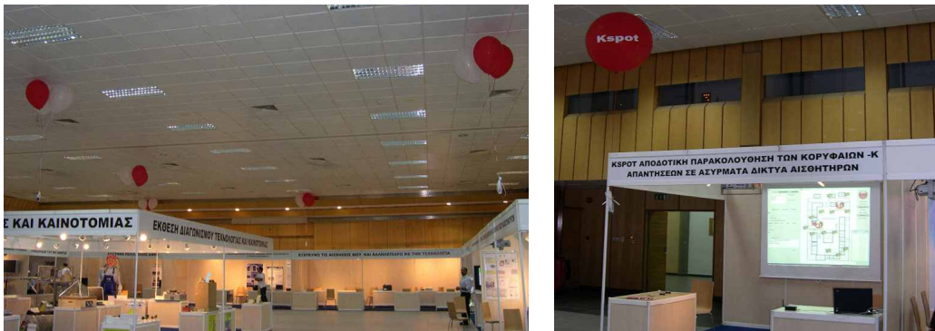
Figure 2: KSpot + 's prototype implementation deployment during the event “Researcher’s Evening” at the Cyprus International Fair in 2009. (Left) Sensor nodes were placed over the pavilions using helium balloons. (Right) Sink station was connected with a laptop computer that projected the pavilions with the highest noise level.
